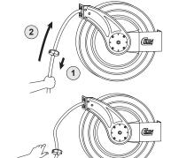
To unlock the hose when you have finished using it, (1) simply pull it out a small distance and listen for the latch to stop "clicking".
